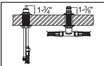
(2) Confirm the valve and spout dimension for 1-3/4" & 1-3/8" where 1-3/4" is the required valve height from the finished deck. And 1-3/8" is the shank height from the finished deck.
