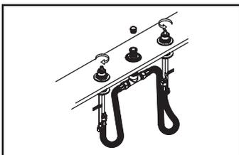
(1) Remove the mud guards from the spout shank and valves. Remove test cap from spout shank.
