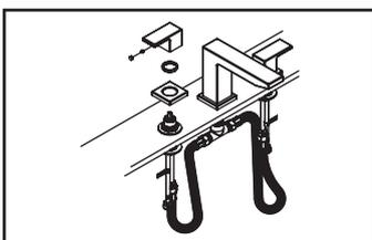
(4) Place valve escutcheon on both side valves. From top of valve escutcheon, thread sleeve on valve to secure valve escutcheon. Ensure handles move in correct direction; tighten Allen screw with help of Allen Wrench tool provided to install both side handles. Turn on both side handles to check for any leaks.
