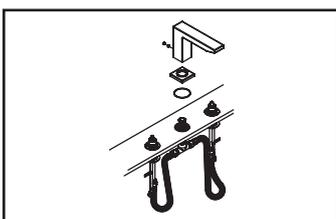
(3) Place the washer underneath of the spout escutcheon. Carefully slide the spout on the spout shank so the o-ring on the spout shank does not get damaged. Tighten the 1/8" Allen screw with the help of the Allen wrench tool provided. Do not overtighten. Place the hole cover to cover the hole.
