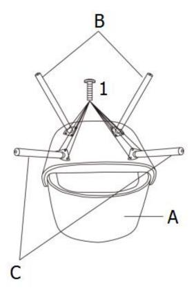
Attach the Front Legs (B) and Back Legs (C) to the Seat (A) with Allen Key Screws (1). Use Allen Key (2) to tighten.
