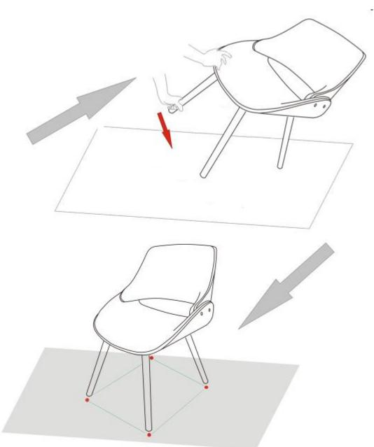
Place Chair on a flat level surface to ensure it is level. If the Chair is uneven, adjust the uneven leg slightly to make it level.
