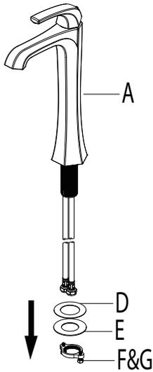
Shut off the water supply. Remove the old faucet. Clean the mounting surface. Remove the mounting nut & screws (F&G), metal washer (E) and plastic washer (D) from the faucet (A).
