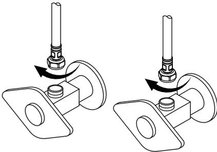
**NOTE:** Please make sure filter washers are installed before connecting to the main valve.
