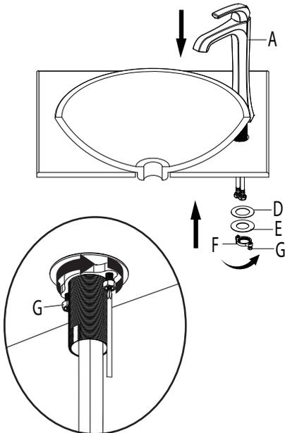
Place the faucet (A) through the hole in the countertop. Secure the faucet (A) to the countertop using the plastic washer (D), metal washer (E) and mounting nut (F) provided. Tighten screws (G).
