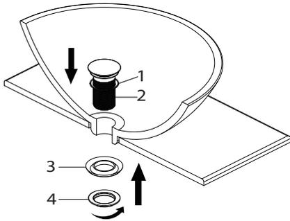
Place the washer (1) underneath the flange of the pop-up body (2). Slide the pop-up body (2) down through the drain hole on the vessel or basin sink. From the underside of the sink, slide the washer (3) against the bottom of the vessel or basin sink, thread on the coupling nut (4) and tighten. Do not overtighten.
