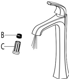
After installing the faucet, remove the aerator (B) with the included aerator key (C). Turn the water on for 30 seconds to remove any debris. Reassemble the aerator (B).
