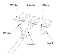
Connect black input wire to black fixture wire. Connect white input wire to white fixture wire. Connect green ground wire (may be bare copper) to green fixture wire.
