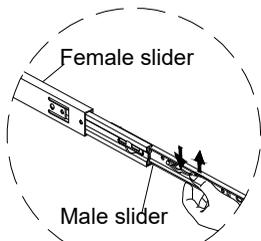
**Schematic diagram of slide rail disassembly**
