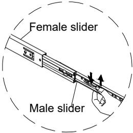
Schematic diagram of slide rail disassembly
