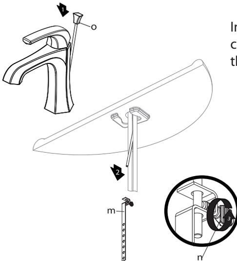
Insert lift rod (o) through spout and connect with extender rod (m). Tighten thumb screw (n).
