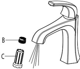
After installing faucet, remove aerator (B) with included aerator key (C). Turn water on for 30 seconds to remove any debris. Reassemble aerator (B).
