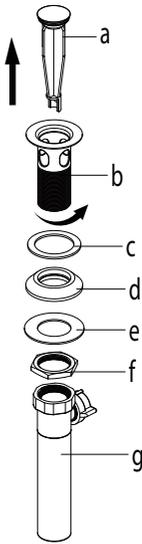
Remove waste stopper (a) and drain flange (b) from tailpipe (g). Remove concave washer (d), metal washer (e) and mounting nut (f) from drain flange (b).
