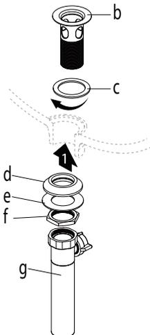
Insert drain flange (b) through drain hole with rubber washer (c) attached. From underneath, place concave (d) and metal washer (e) on drain flange. Secure with mounting nut (f). Thread tailpipe (g) onto drain (b) and hand tighten.
