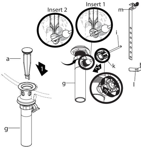
Insert waste stopper (a) into drain flange. Remove extender rod (m) and clip (l) from drain off pole (i). Remove nut (k). Insert drain off pole (i) into drain pole opening of tailpipe (g). See insert 1. Secure nut (k) to drain off pole opening of tailpipe (g).
