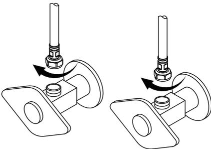
Attach waterlines to angle stops
