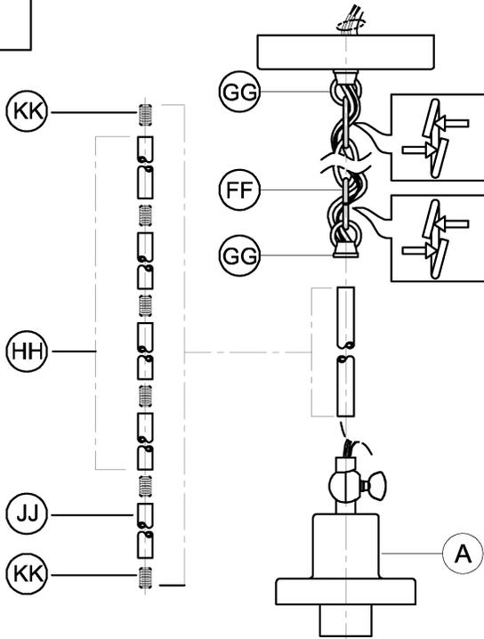
3. Pass the wires through the one pipe (JJ)/nipple (KK)/four pipes (HH) and chain loop (GG) to achieve overall desired length. Next attach pipes onto fixture (A) to secure tightly. Weave electric cord and ground wire through chain (FF) and canopy (D). Open two links of chain and attach both ends to chain loops (GG). Close the chain links.
