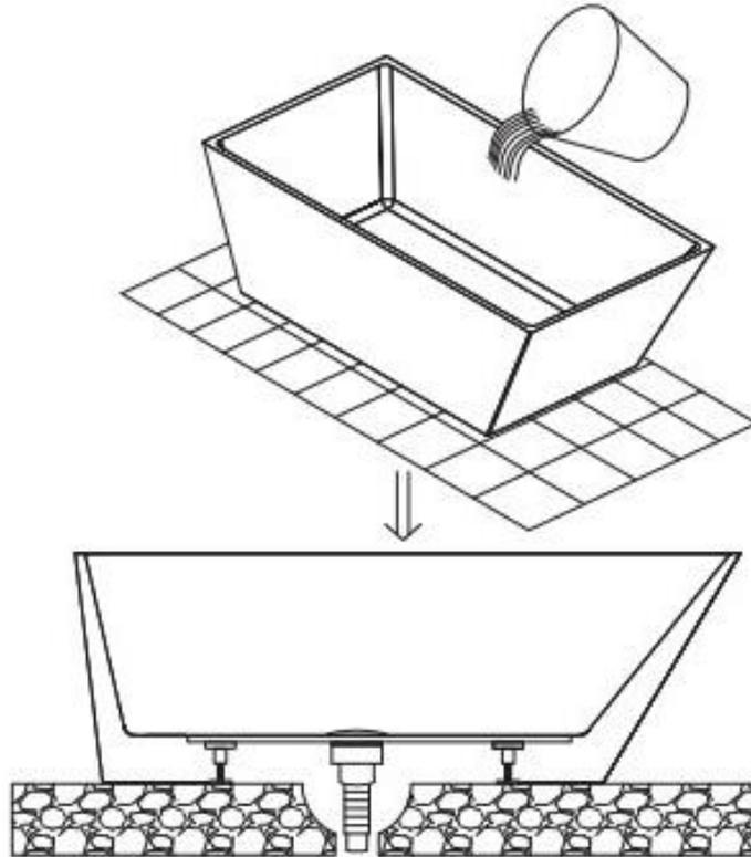
**2-5. Apply a thick layer of silicon sealant around the bath outline allow it set 24 hours.**
