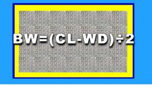
Add up the combined length of the full tiles. Subtract this distance from the wall dimension and divide the result by 2.
