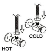
5. Attach flexible hose to water supply.
