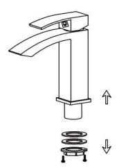
1.Remove the rubber washer, metal 2.Screw and hand tighten the hot and washer and locking nut from the faucel.
