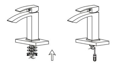
3.Install faucet through center hole. 4.Re-install the rubber washer followed by the metal washer and lock—nut.Hand tighten then tighten further using a screw driver to tighten lock nut screws.
