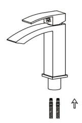
cold flexible hoses to the faucet. Do not use a wrench to tighten hoses as this may damage the hose and/or the hose threads.
