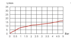
Test pressure: 1.6MPa (16bar) Flow pressure: Min 0.05MPa Max 1.60MPa Recommended pressure: 0.1MPa to 0.8MPa (1 to 8 bar)
