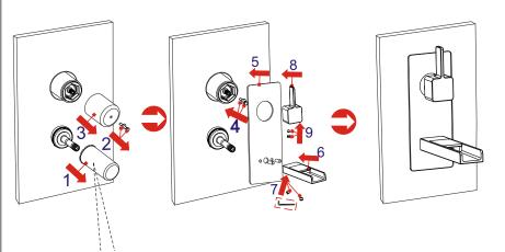
After installing the main body, read the index on cover, install the decorating tiles and glue the plate (5).
