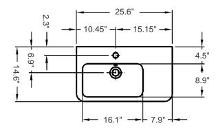
All dimensions are nominal Faucet and drain fittings not included. Shown only for photographic purposes. The 3/8" Hot & Cold water-supply tubes and 1-1/4" P-trap outlets are variable and can be determined at the discretion of the installer
