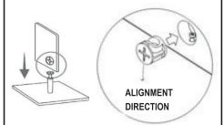
3. The panels might have a very small gap which is normal; turn the cam lock clockwise to lock the parts together and the gap will also close.
