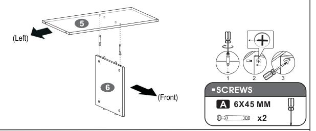
Assemble the right back panel ① to panel ⑤ using bolts as shown and as explained in page 3.
