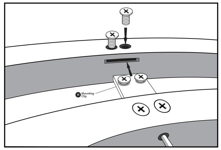
Remove last two screws from mounting clip (H). Insert mounting clip (H) into slot on ring frame. Secure ring frame and mounting clip (H) with screws.
