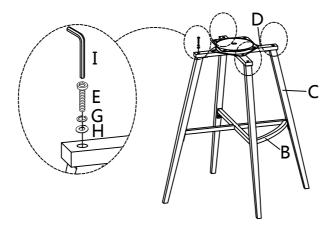
Attach Rotary Turntable (D) to the bottom of Chair Seat (A) using Long Bolt (E), Spring Washer (G), Flat Washer (H) with Allen Key (I).
