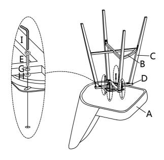
With assistance from your adult partners, turn the Chair right way up. Adjust the pre-installed levelers on the bottom of Leg (C) until the Chair is level with the ground.
