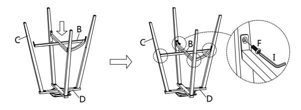
Stand the metal base up. Use Long Bolt (E), Spring Washer (G), Flat Washer (H) with Allen Key (I) to fix Rotary Turntable (D) and Leg (C).
