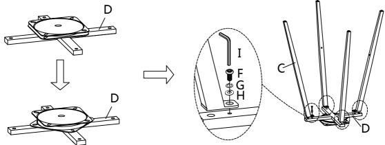
Put Leg Support (B) between assembled leg frame. Use Bolt (F) with Allen Key (I) to fix Leg Support (B) and Leg (C).
