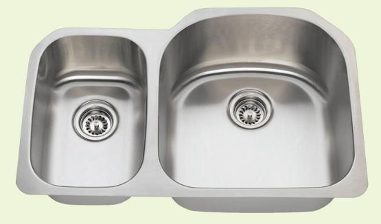
31 1/2" x 20 7/8" x 9 1/4" 16- or 18-Gauge Steel Available Certified High-Quality 304 Stainless Steel **Brushed Satin Finish** Offset Drain Thick Sound Dampener Rubber Pad Fully Insulated **One-Piece Construction** Cardboard Cutout Template Included Installation Hardware Included cUPC Certified (Uniform Plumbing Code) Limited Lifetime Warranty
