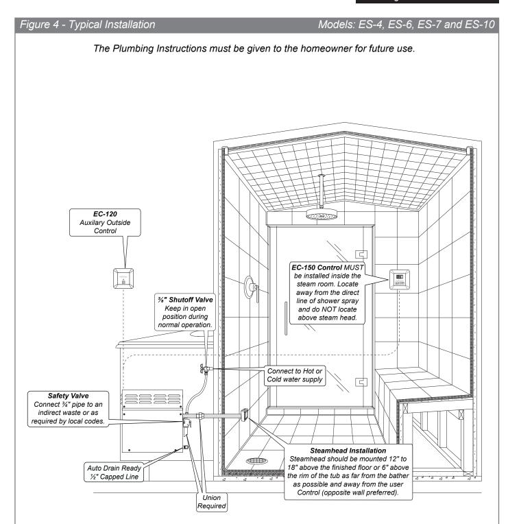
Steam Outlet Pipe - Use a 3/4" Copper or Brass pipe.
