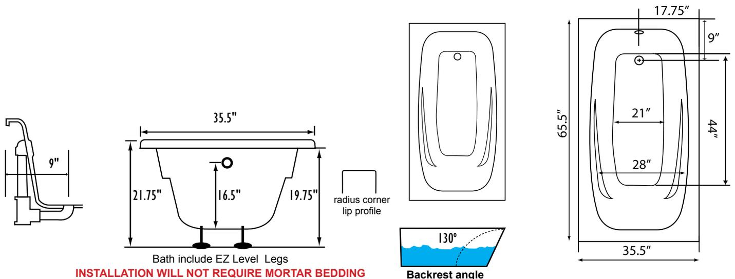
Some standard & most alternate pump locations may stickout past perimeter of the bath 1"-3". NOTE: Graphics may not be to scale. Specifications and features are subject to change without notice and are  $\pm .25"$ . All final measurements should be taken from tub on site. Access 18"x 18" or larger is required for each pump. Consult your contractor for installation requirements.
