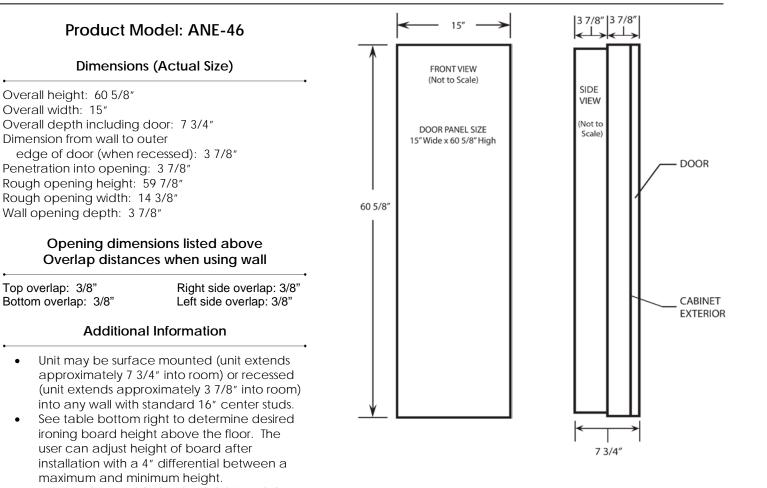
Unit can be provided with a left hinged door • upon request. Right hinge is standard.
