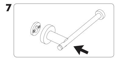
Place the toilet paper holder over the mounting plate with the set screw on the bottom.
