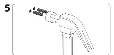
Insert provided anchors if mounting into drywall. Anchors not necessary if mounting into wood studs.
