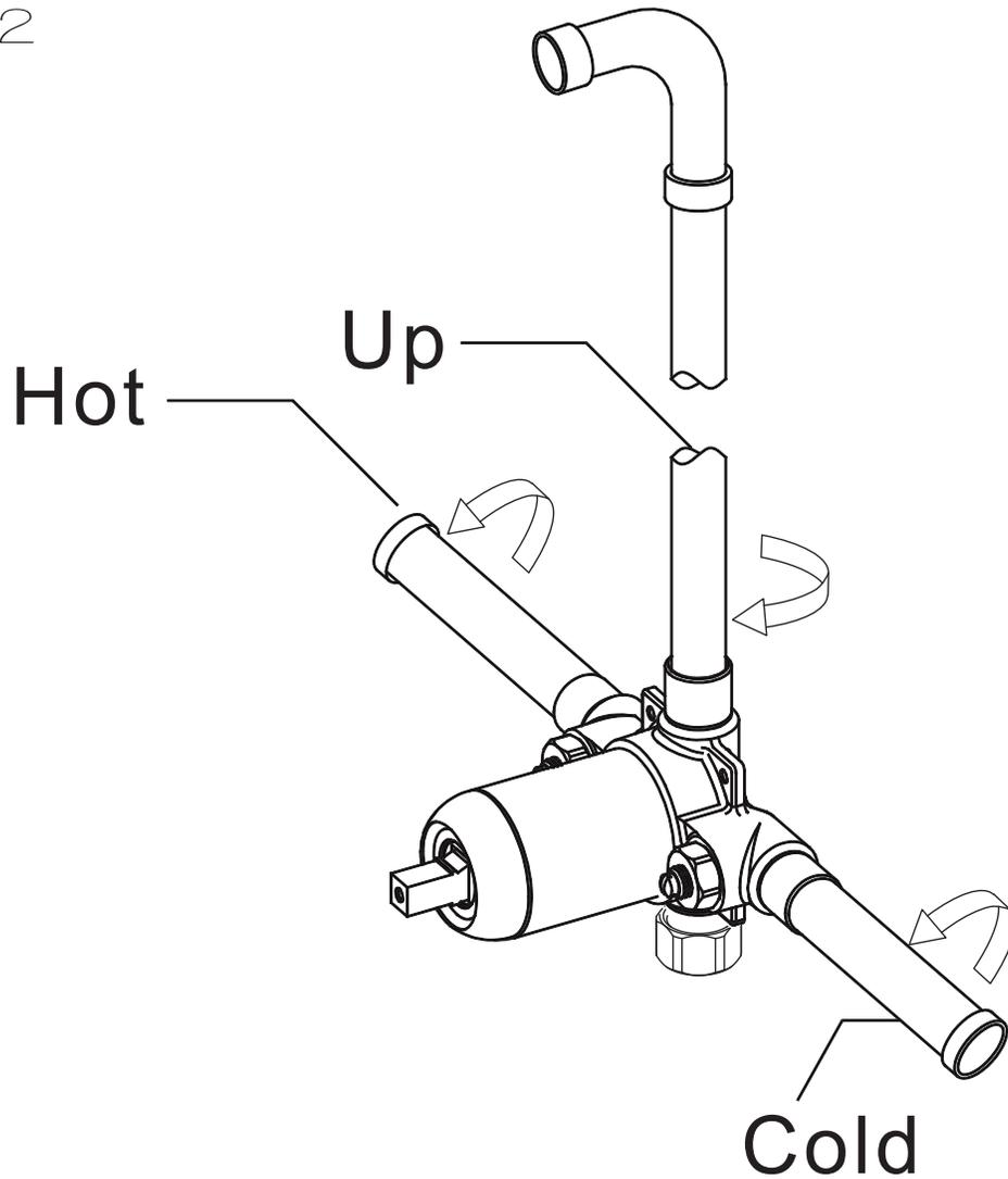
**Step 2A** Connect all plumbing lines to the faucet valve as shown.
