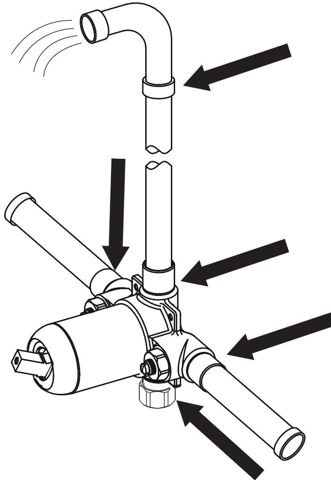
**Step 3A** Turn on water and allow it to run for 1-2 minutes.
