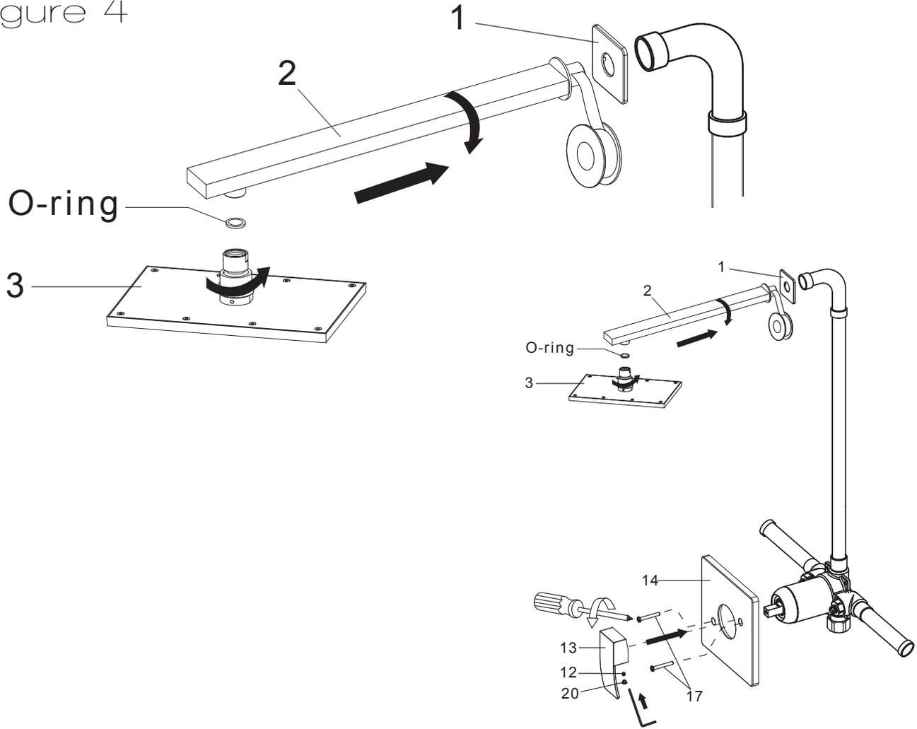
**Step 4A** Apply Teflon tape to the shower arm (#2) then place shower arm flange (#1) on shower pipe and screw shower arm to the pipe.
