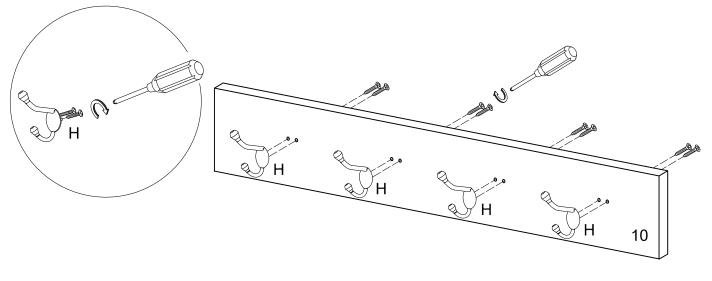
Disassemble screws from hook, then attach hook (H) to part (10) using screw with screwdriver.
