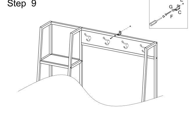
Secure furniture to anchor in wall using washer (G) and screw (F) with a screwdriver.
