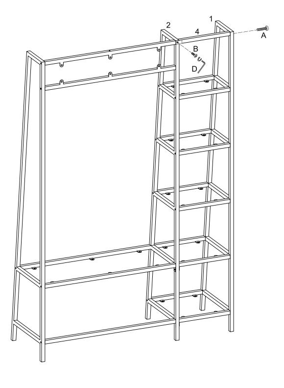
Attach part (4) to part (1,2) using bolt (B) with hex key (D).
