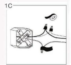
Tape wires and wire nuts together using electrical tape.
