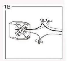
Strip 3/4" of insulation from wire ends. Connect house ground wire to fixture ground wire. Twist wires together using wire nut. Connect the black house wire to the smooth or black fixture wire. Twist wires together using wire nut. Connect the white house wire to the ribbed or white fixture wire. Twist wires together using wire nut.
