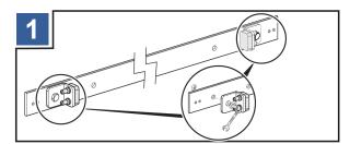
Before beginning installation, attach the door stops [C] to the rail [L].
