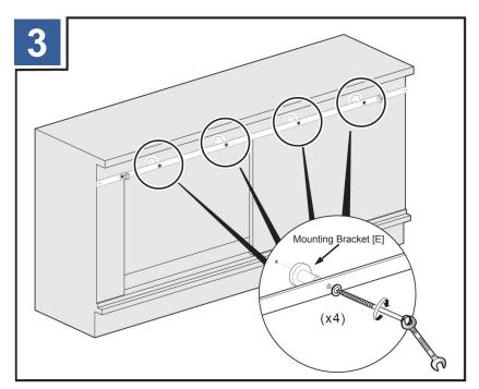
Install the rail, and mounting brackets [E].
