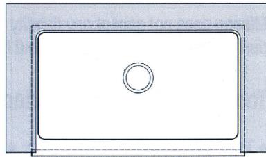
Built-up installation may expose sink sides to be raised up to 1" above the countertop.
