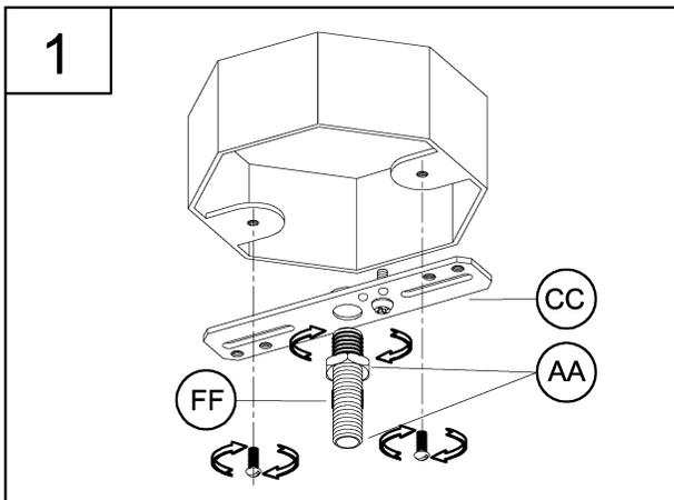
1. Loosely thread the hex nut (AA) onto the nipple (FF) and then install this assembly onto the mounting strap (CC). Next, install this assembly to the outlet box using the mounting screws supplied with the outlet box (not included).
