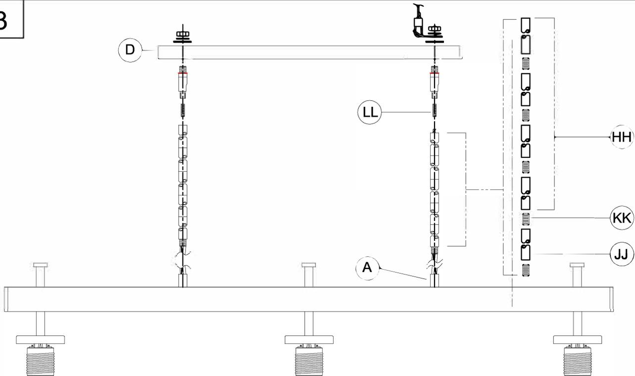
**NOTE:** During this step, determine the hanging length of your fixture by adding or removing pipes. The electrical and ground wire may also optionally be cut to length. Remove the swivels if they are already assembled to the canopy. You will re-assemble them onto the top of the last pipe before wiring has been passed through during this step. Align them so they will swivel in the same direction.
