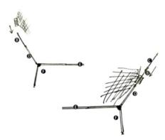
6. Hook the upper loop of the net G) to the top of upper fiberglass rod(C). Do this in both sides.
