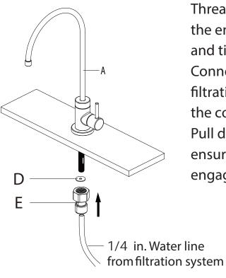
Thread the quick connect adaptor (E) onto the end of the faucet assembly (A) stud, and tighten securely using a wrench. Connect the water line from the filtration system by pushing the line into the connector (E).
