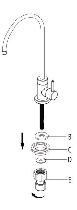
Remove the rubber washer (B), ABS mounting (C), rubber washer (D) and connector (E) from the end of the stud.
