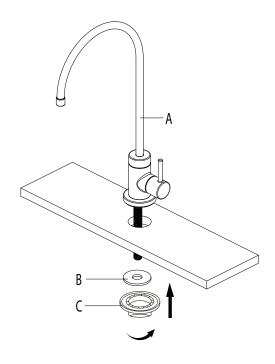
Place the faucet assembly (A) through the selected hole in the sink or countertop. On the underside of the sink or countertop, slide the rubber washer (B) and ABS mounting (C) onto the stud. And tighten securely using your wrench.
