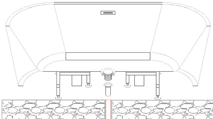
6. Flip the tub over and carefully set the tub into position with tail piece assembly to P-trap and connect to the drain.
