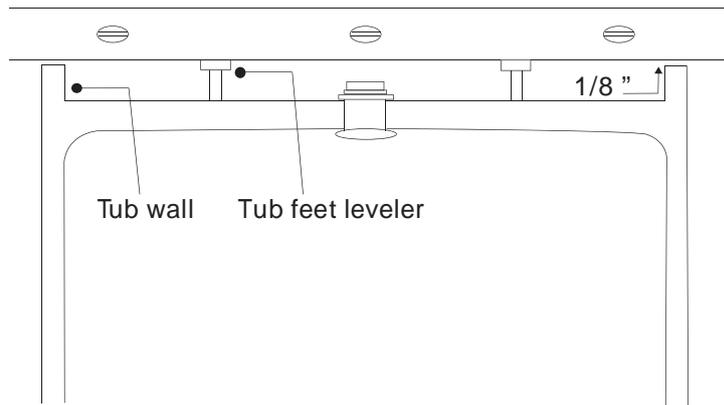
3. Place a level across the bottom of the tub and adjust the tub feet leveler to touch the level. Then raise the leveler additional 1/8" or 3/16" so that the weight of the tub, water and user are fully supported by the feet adjuster and not the tub walls.
