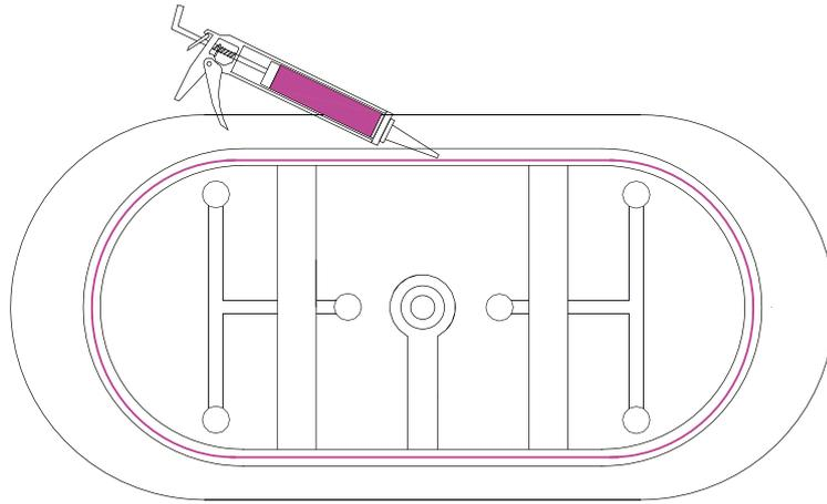
5. Apply a generous bead of adhesive or waterproof silicone to the bottom of the tub and a bead of tub and tile caulk around the edge of the tub
