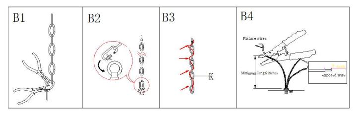
Step B1: By measuring, determine the correct length of links needed. Use the chain pliers, cut and discard the remaining links.
