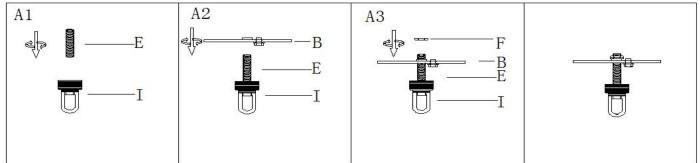
Step A1:Thread the nipple(E) into the screw collar loop (I)
