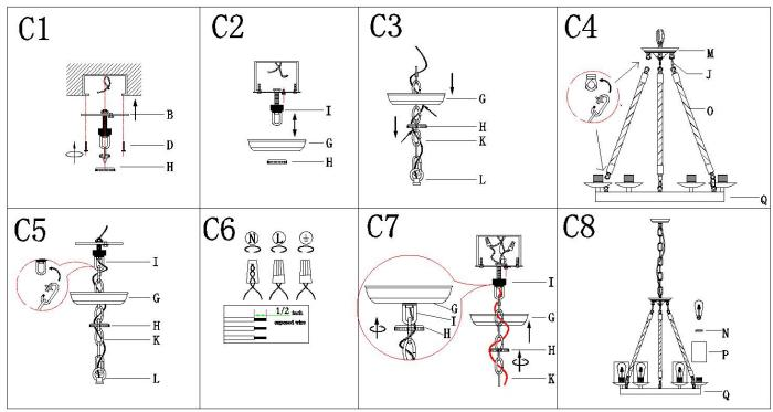
Step C1: .Attach single bar (B) to outlet box with mounting screws (D). The side of single bar marked "GND" must face out Step C2: Raise the canopy (G) through screw collar loop (I) and screw the collar loop (I) to a proper position by measuring .
