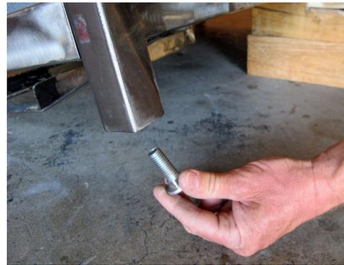
5. Set your Impact Fire Table in place on a flat, solid surface and make necessary adjustments to the adjustable feet so the top surface of your fire table is level.
