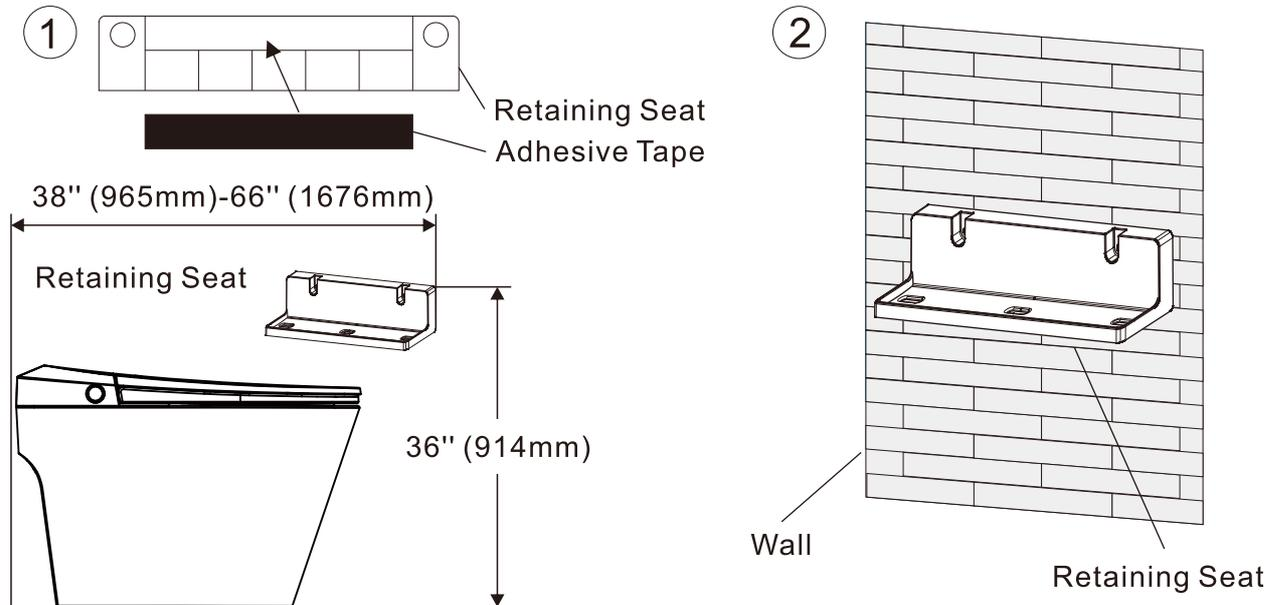
Select the smooth and even position of the remote control retaining seat. Tear off one side of the double-sided adhesive tape and stick it on the back of the retaining seat.
