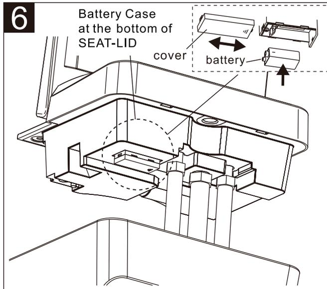
1. Carefully remove the cover of the battery case.
