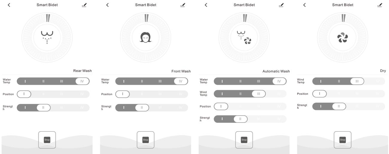
1. On this page, you can adjust the water temperature, wind temperature, nozzle position, water pressure intensity.
