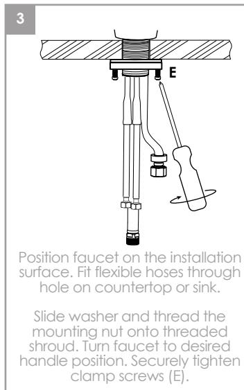
Position faucet on the installation surface. Fit flexible hoses through hole on countertop or sink.
