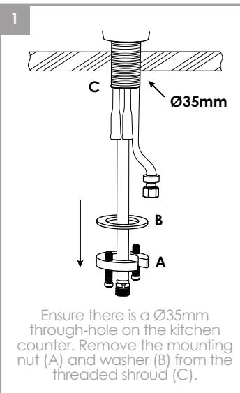
Ensure there is a Ø35mm through-hole on the kitchen counter. Remove the mounting nut (A) and washer (B) from the threaded shroud (C).
