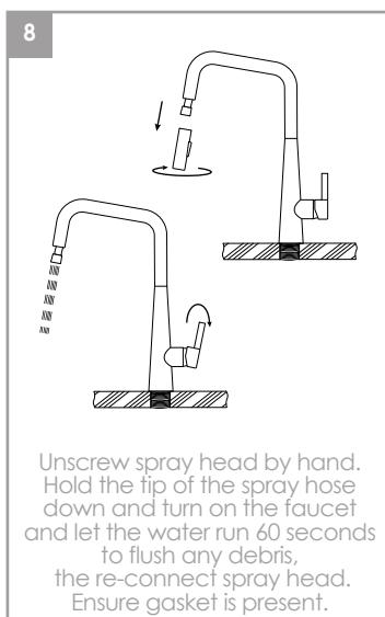
Unscrew spray head by hand. Hold the tip of the spray hose down and turn on the faucet and let the water run 60 seconds to flush any debris, then re-connect spray head. Ensure gasket is present.
