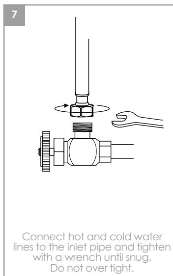
Connect hot and cold water lines to the inlet pipe and tighten with a wrench until snug. Do not over tight.
