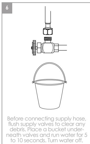
Before connecting supply hose, flush supply valves to clear any debris. Place a bucket underneath valves and run water for 5 to 10 seconds. Turn water off.
