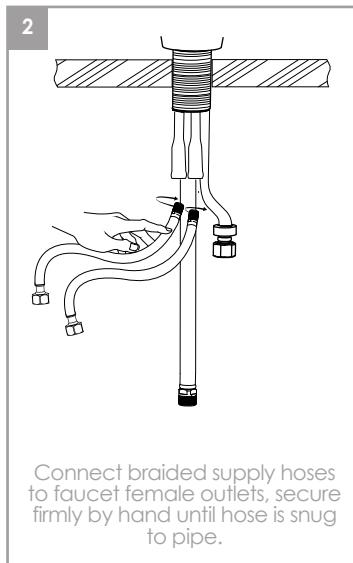
Connect braided supply hoses to faucet female outlets, secure firmly by hand until hose is snug to pipe.
