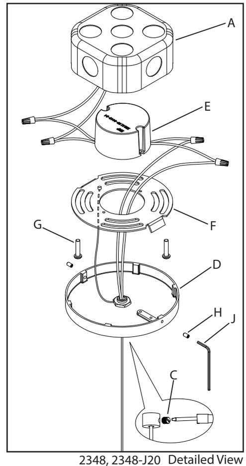
1. Shut off power to the outlet box (A).
