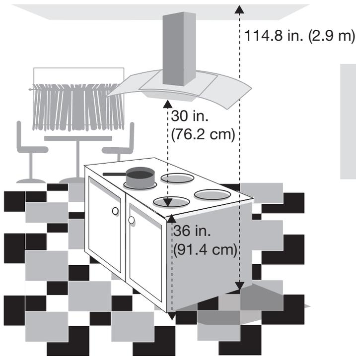
Maximum ceiling clearance 114.8 in. (2.9 m) at 30 in. (76.2 cm) hood mounting height above countertop or stove (May vary with different model). Chimney extensions available for higher ceiling.
