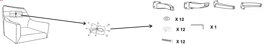
Step 2. Using bolts (H3), lock washers (H2), flat washers (H1), connect Front Legs (P2)(P3) and Back Legs (P4)(P5) to Chair (P1). Tighten bolts (H3) with Allen Wrench (H4).
