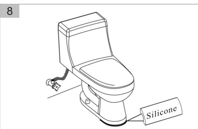
8. Install water closet seats according to the installation instruction, then daub a layer of silicone between the product and floor.
