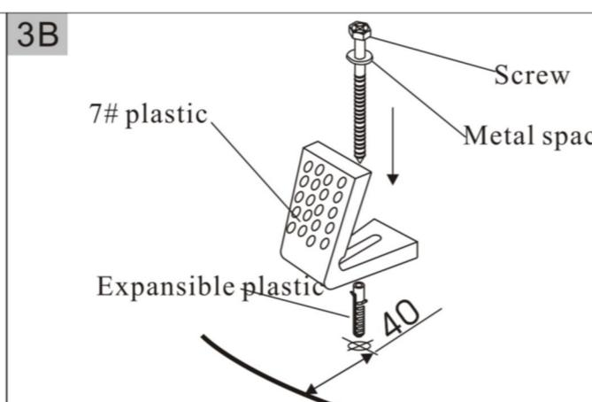
3. Remove the product and drill holes according to the marks. Then insert the plastics.
