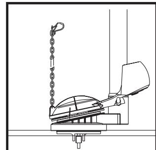
Screw the flush valve tight, and make sure the fixture block and seal washer attach on the tank wall. Put the flapper on the flush valve .
