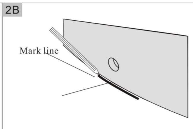
2. Put the water closet onto the installing position. Make sure the + centre lines of floor and water closet are aligned. Then mark the installing holes with pencil.
