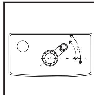
Adjust the angle of the flush valve, make sure the flapper is easy to open, and the chain is not blocked.
