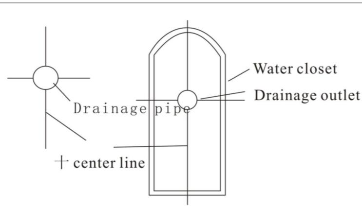
1. Mark the + centre line according to the drainage outlet on the floor and the one of the water closet.
