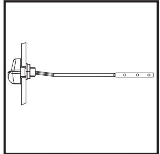
Enter the nut on the handle and tighten.
