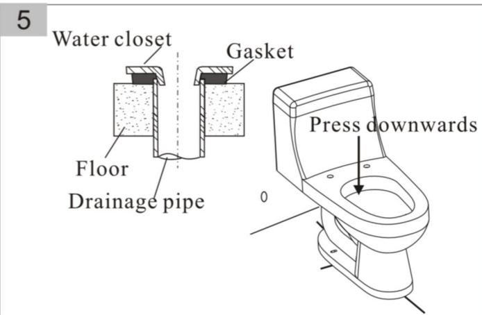
5. Clean the drainage outlet, then put up the water closet to make the centre line of it aligned with the one on floor and the centre of waste outlet aligned with the centre of drainage outlet. Press downwards the product until it is flat.
