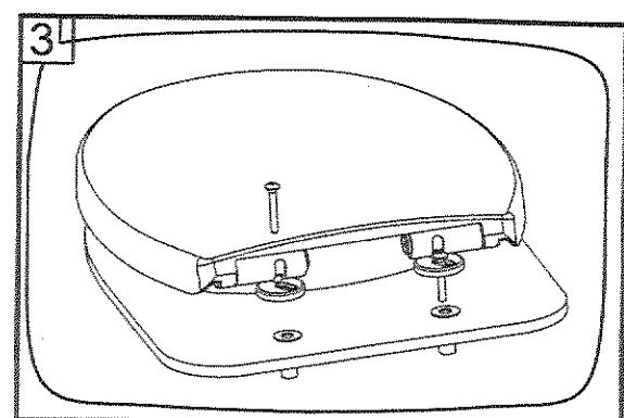
Plug the bolt into the expansion rubber.
