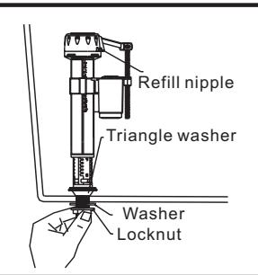
Unscrew the locknut and washer. Position the fill valve into the tank, then screw the washer and locknut.
