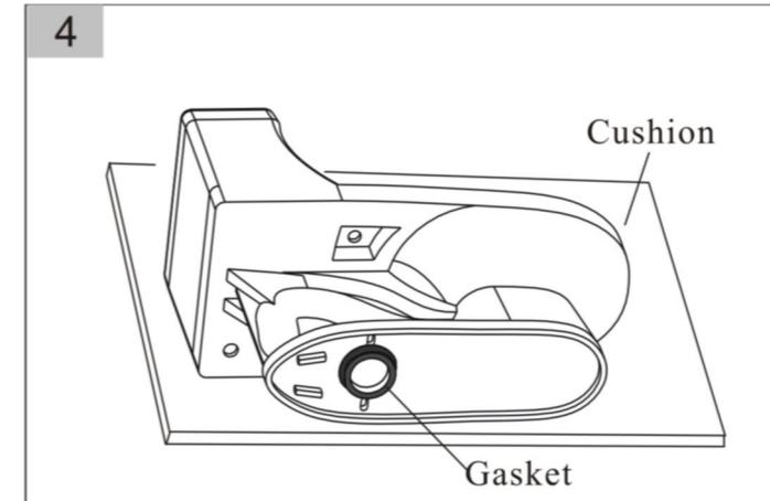
4. Put the product onto the cushion flatly, then cover the gasket onto the drainage outlet tightly.
