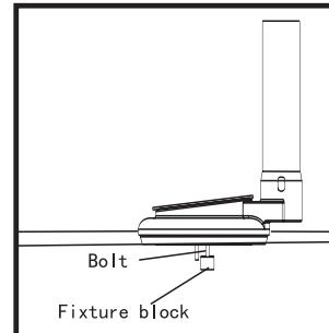
Screw the flush valve tight, and make sure the fixture block and seal washer attach on the tank wall. Put the flapper on the flush valve .
