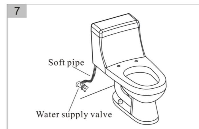
7. Install the water supply valve, then connect the filter and water supply soft pipe of cistern. Check the connection carefully to make sure there is no leakage.
