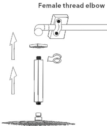
1. Connect shower arm with the cover before screwing arm into riser connection to prevent damage.
