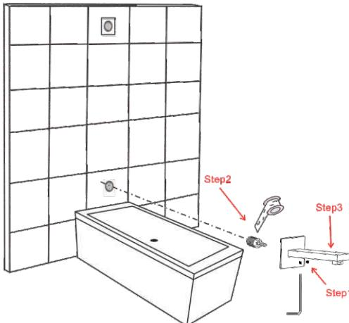
Step 1: Remove the screws at the bottom of the bathtub faucet and detach the copper connector.
