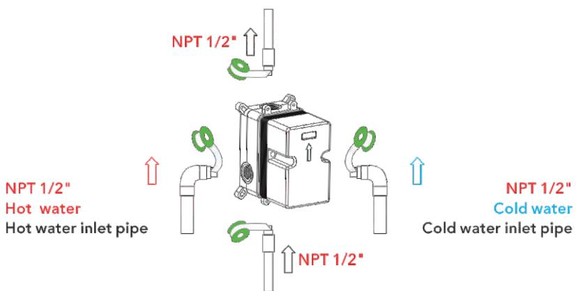
1. As shown in the figure, the inlet and outlet pipes are pre-buried. Please pay attention to the correct direction when installing the pre-buried main body.
