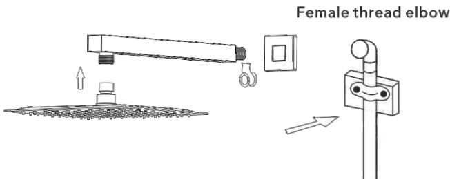
1. Connect shower arm with the cover before screwing arm into riser connection to prevent damage.
