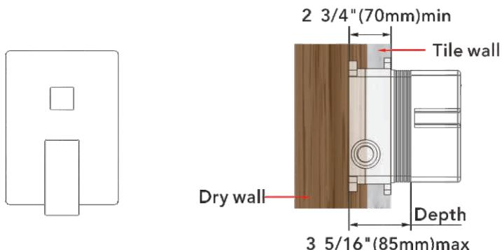
Notice: 1. The installation depth of the main body should be no less than 2 3/4" (70mm) and no more than 3 5/16" (85mm), including the thickness of the tile. Otherwise, the deck plate cannot be installed.
