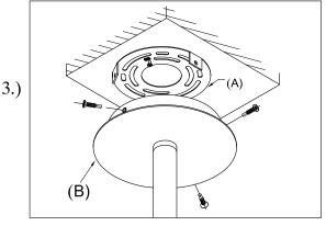
Step 3: Attach the body (B) to the mounting bracket (A) using three screws provided.
