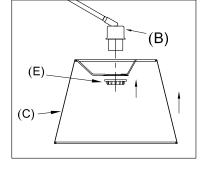
Step 4: Remove the socket ring (E) from fixture (B). Attach shade (C) and secure using socket ring (E).
