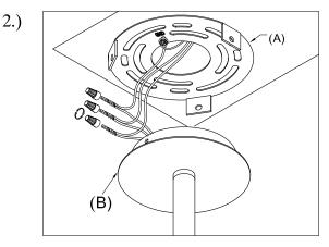
Step 2: Wire fixture to wires in outlet box. Copper wire is for ground
