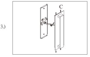
Step.3: Caulk around fixture with outdoor silicone sealant to prevent water intrusion.
