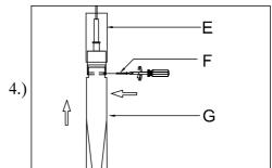
Step 4: Attach glass (G) using set screws (F).
