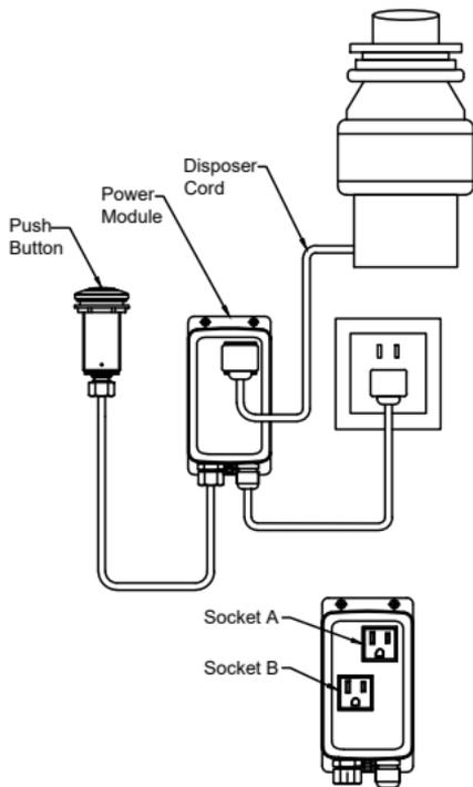
Plug the disposer cord in the power module.
