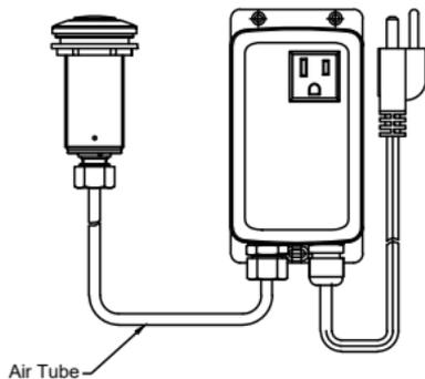
Attach air tubing between the push button and power module.
