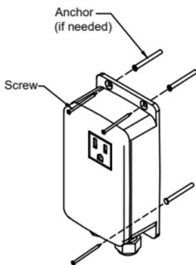
Mount the power module to the cabinet wall atleast three feet within an electrical outlet and the disposer.
