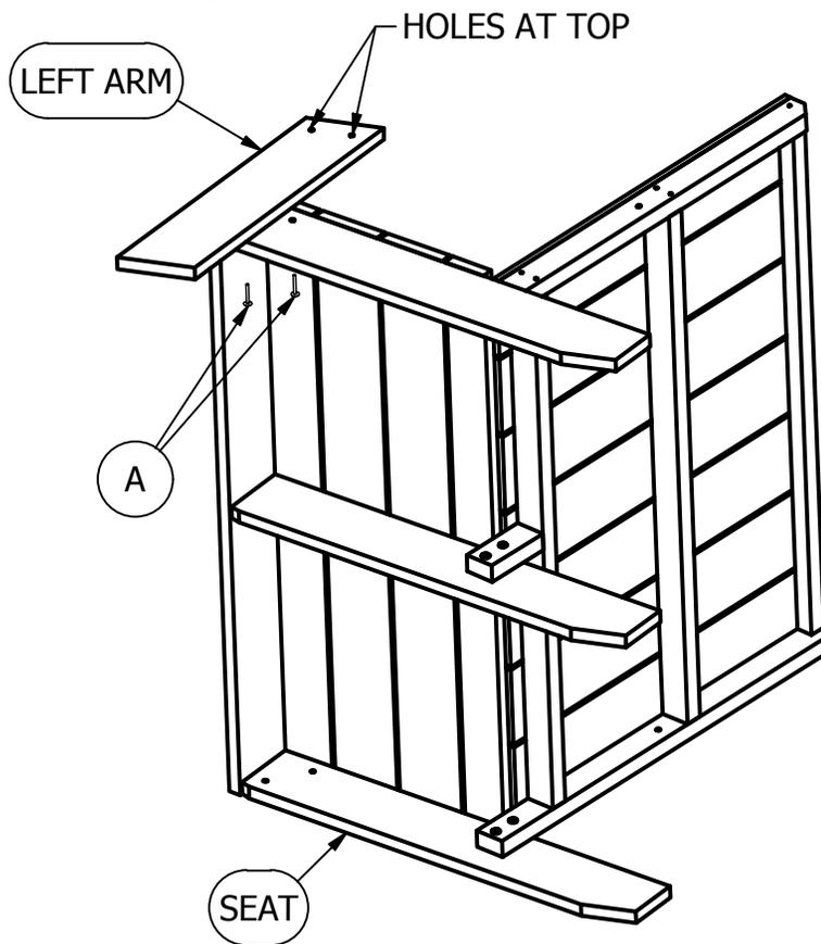
**2)** With Holes Positioned at the Top as Shown, Attach Left Leg to Seat Using (2) "A" Bolts.
