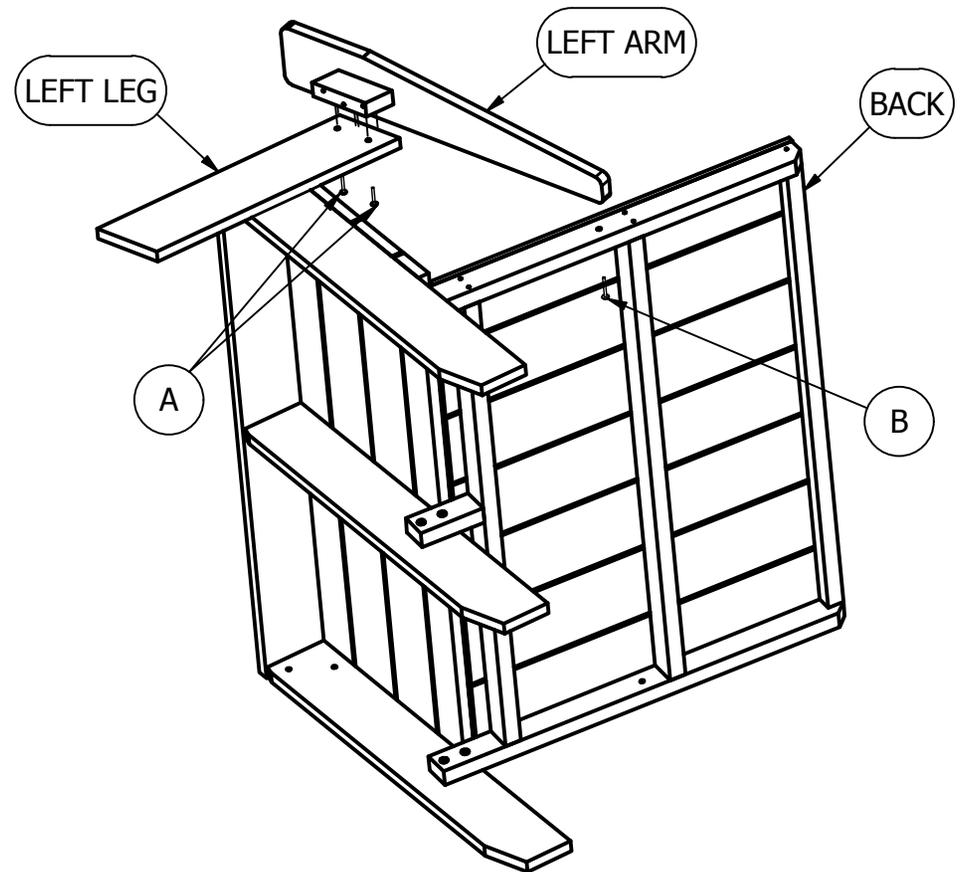
**3)** Attach Left Arm to Left Leg Using (2) "A" Bolts. Attach Left Arm to Back Using (1) "B" Bolt.
