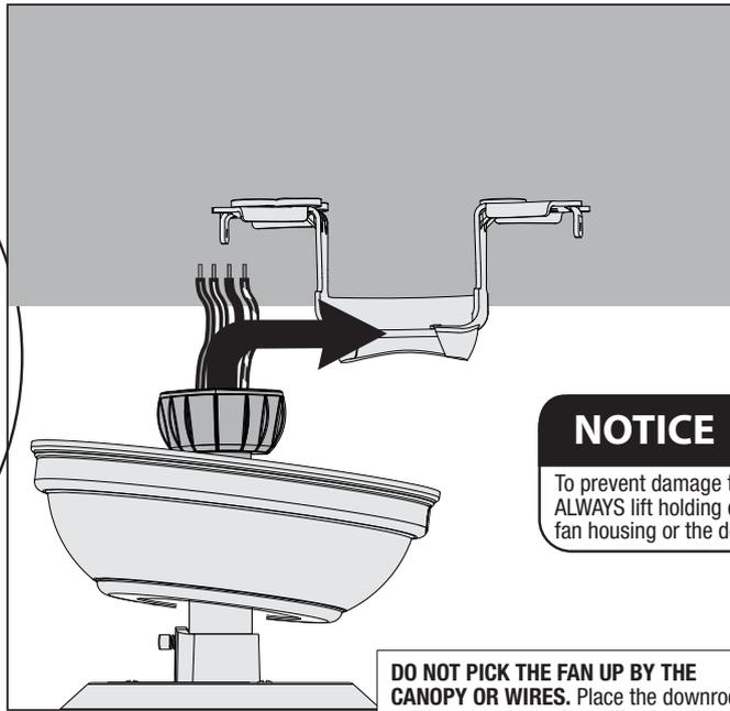
**DO NOT PICK THE FAN UP BY THE CANOPY OR WIRES.** Place the downrod ball into the slot in the ceiling bracket.
