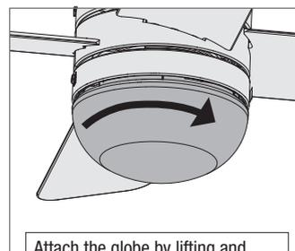
Attach the globe by lifting and turning clockwise one third of a full turn of the glass until it stops.
