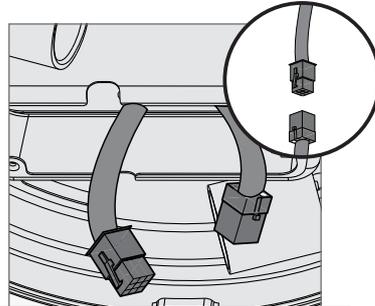
Feed the 9-pin plug connector coming from the bottom of the motor housing through the center hole in the light kit assembly. Connect it to the plug connector found in the switch housing area of the light kit assembly. Make sure to line up the colored markings on the connectors.
