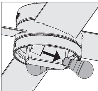
Install the included bulbs into the sockets. When necessary, replace with bulbs of same wattage.
