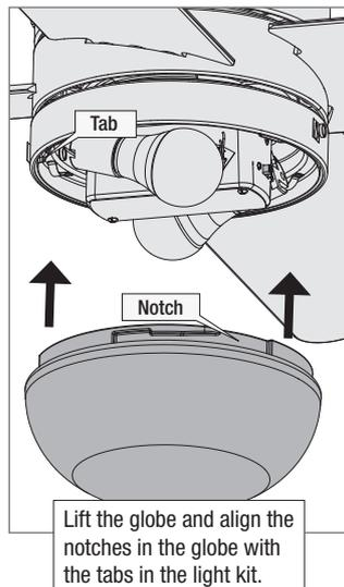
Lift the globe and align the notches in the globe with the tabs in the light kit.
