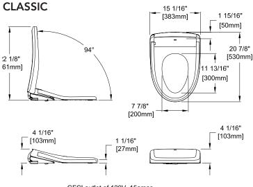
GFCI outlet of 120V, 15amps. Power cord is 4' long with 3 prongs.
