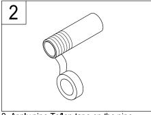
Apply pipe Teflon tape on the pipe nipple threads.
