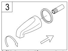
3. Slide the spout and flange over the pipe. With the spout tight to the wall, tighten the set screw to the pipe.
