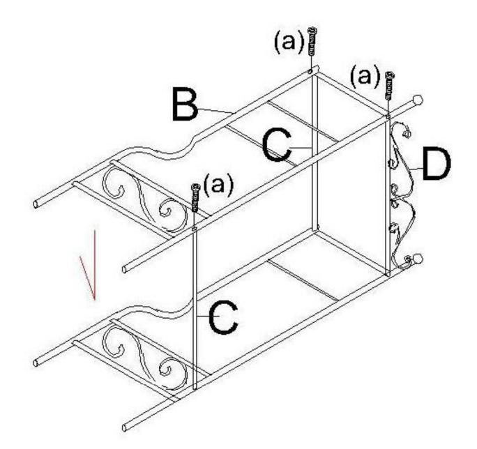
NOTE: Place this unit on the floor to check if it is stable before tightening Bolts (a).
