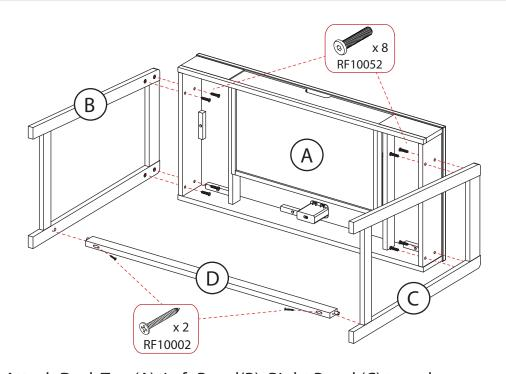
Attach Desk Top (A), Left Panel(B), Right Panel (C) together by using screw (RF10052). Attach Crossbar (D) to (B) and (C) by using screw (RF10002) as per diagram.
