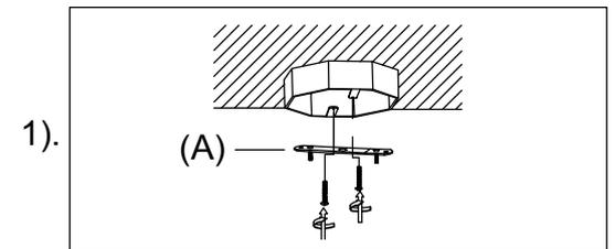
Step.1: Remove mounting bracket (A) from fixture and install to electrical box.
