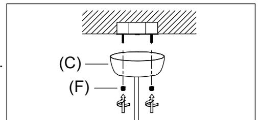
Step.4: Install body (B) to bracket (A) and tighten nut (F) on the canopy (C) to secure. Screw glass (E) to the coupling. Install light bulb.
