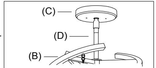
Step.2: Determine correct length of rod needed for hanging height. Screw the Rod (D) on the Body (B) and Canopy (C).
