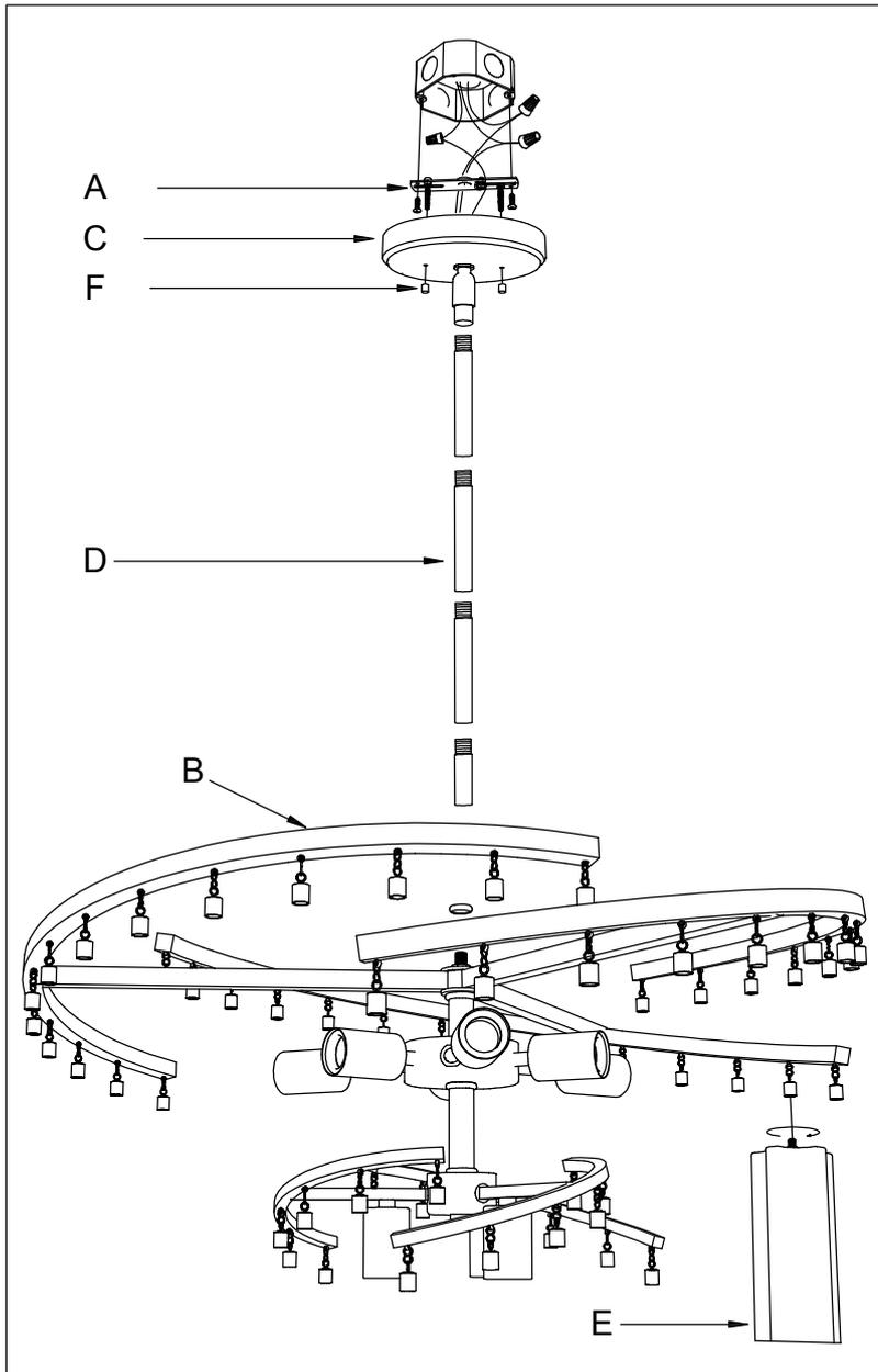
**IMPORTANT: For a safe and secure installation, this fixture must be installed by means of support that is independent of the outlet box.**
