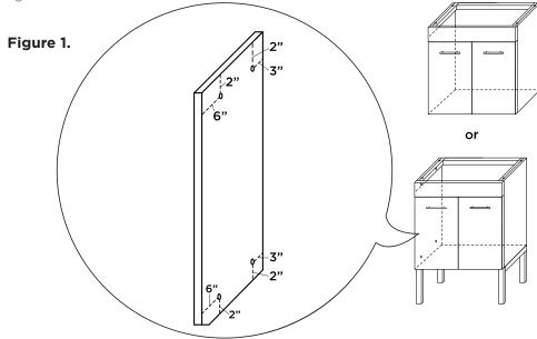
**STEP 2:** Attach drawer bridge to cabinet and secure screws.
